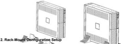
This UPS can be installed into standard 19" rack. It requires the height of 2U from the rack. Use the following procedure to install the UPS into a rack.
