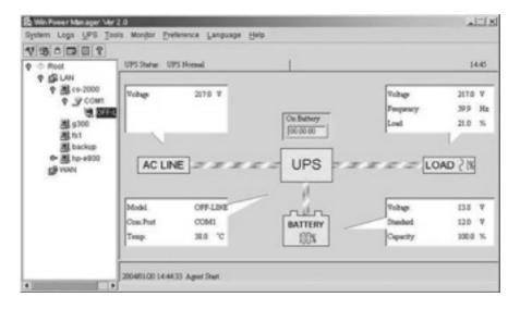
Figure 5. UPS communicates with a computer using WinPower
