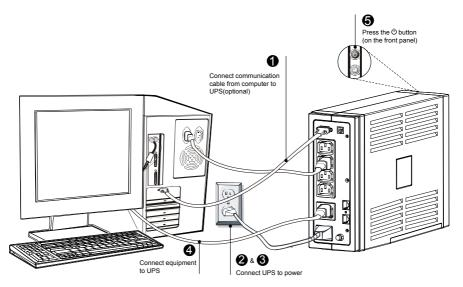
Figure 4. Typical UPS Installation
