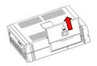
4. Pull the battery out (from bottom side) onto flat area
