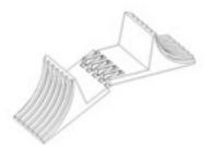
2) Slide down the UPS vertically and put the UPS stands at the bottom of the tower. Then place the UPS into two stands carefully.
