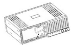
4. Pull the battery out (from right side) onto flat area.
