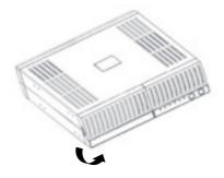
2. Unscrew the battery plate from UPS.
