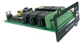
This card provides six output dry contacts and six input contact. These contacts are programmable and user can change the definition for each contact. Please refer to Dry Contact Card manual for more detail.
