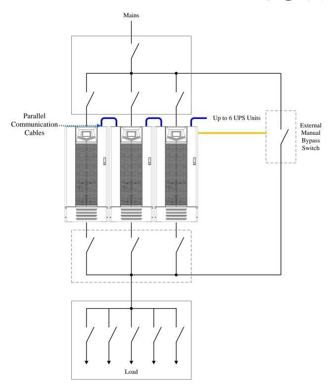
■ Recommended N+1 parallel for dual input system configuration
