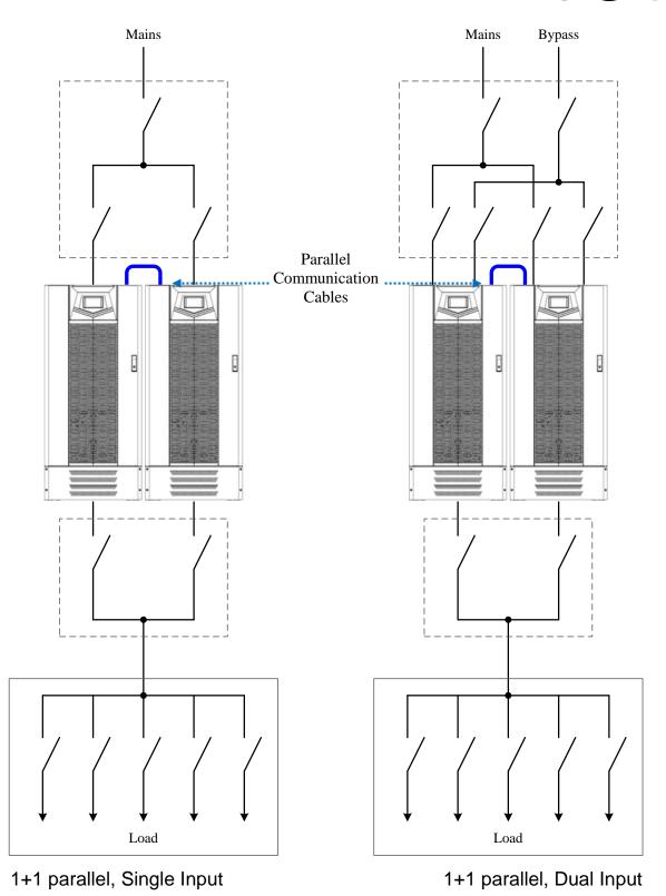
■ Recommended N+1 parallel for single input system configuration
