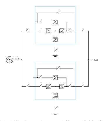
Note: Up to 6 units can be operated in parallel for Converter Mode operation and common battery function is available.
