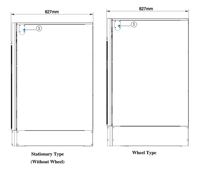
1 Through hole for parallel communication cable
