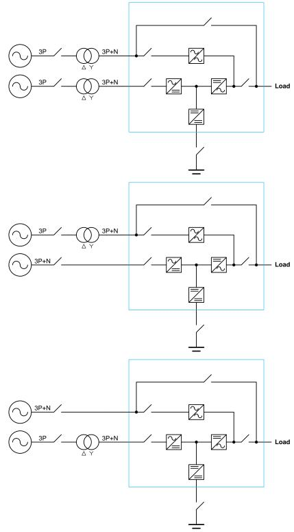
Note: You have to install an isolation transformer on one of the inputs if the two power system are different.
