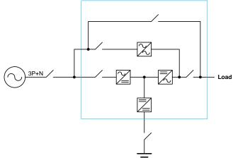
UPS with single input and isolation transformer
