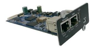
This is Ethernet network card with TCP/IP, HTTP and SNMP protocols.
