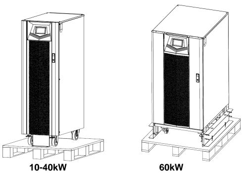
■ Putting 2 fastening rail kits on the pallet edge and making them steady by fastening 4 screws in the pallet.
