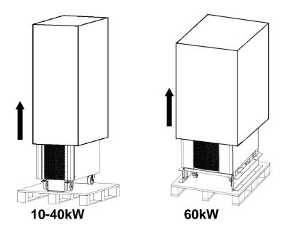
Unscrew the fastening rail kits on the front and rear side of 10-40kW, and right and left side of 60kW.
