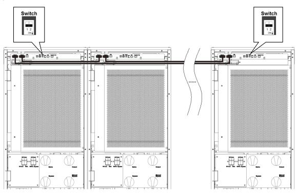
When installing the parallel communication cables, it recommended the parallel communication cable through the hole at side of UPS, as shown below.
