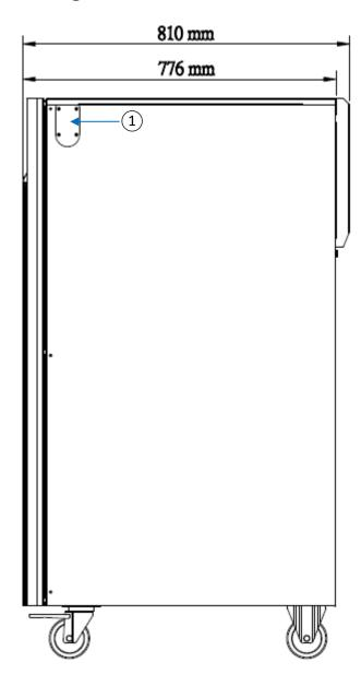
① Through hole for the optional parallel communication cable
