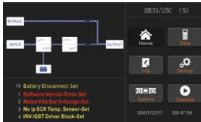
Fig.5-2 Interface of bypass starting
