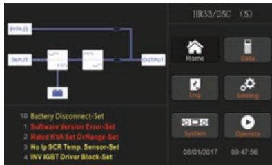
Fig.5-1 Interface of rectifier starting
