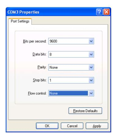
For XP above Windows version, communicate with serial port via serial port debug tool. Double click Putty icon , open Putty and select serial session, configure the correct serial port and baud rate 9600 bps.
